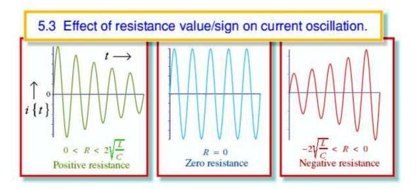
A negative resistance value means that  $\alpha$  is positive. This means the oscillation amplitude and energy grow exponentially with time. In practice, we can't ever obtain an oscillation whose energy grows larger without limit. Infinite powers and energies aren't accessible in the real world! Something always restricts the rate at which the system can 'create' oscillation power. Fairly obviously, this power must also come from somewhere! Negative Resistance Oscillators
